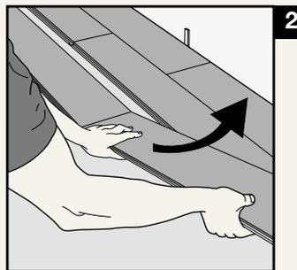
After the whole long side is released you can disassemble each plank by angling the short sides up vertically.
