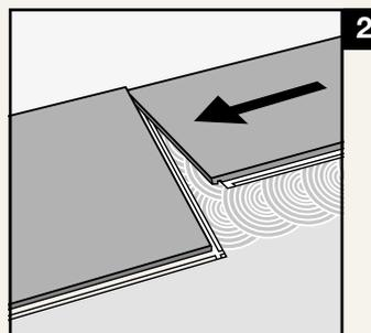
Second plank, first row. Place the plank gently and tight to the short end of the previous plank.
