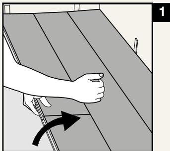
When a plank is locked, it is not possible to take it up by hand. Separate the whole row by carefully lifting up and slightly knocking just above the joint. Fold and release the whole long side.
