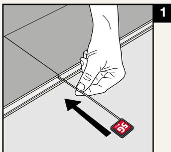
Put the dismantling tool into the space between the tongue and groove on the short end of the plank. Push the dismantling tool forward.
