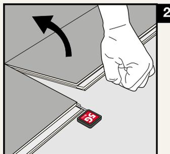
The plank is now loose and you can easily lift the plank up.
