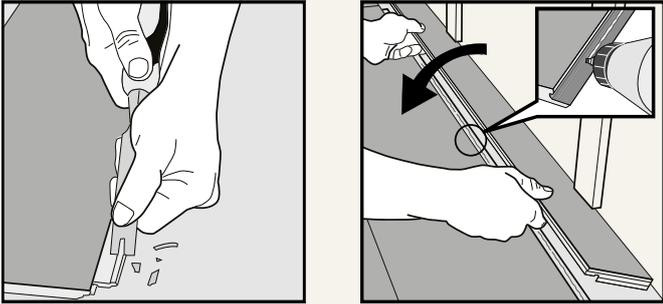
Remove the locking element/hook according to the picture.
